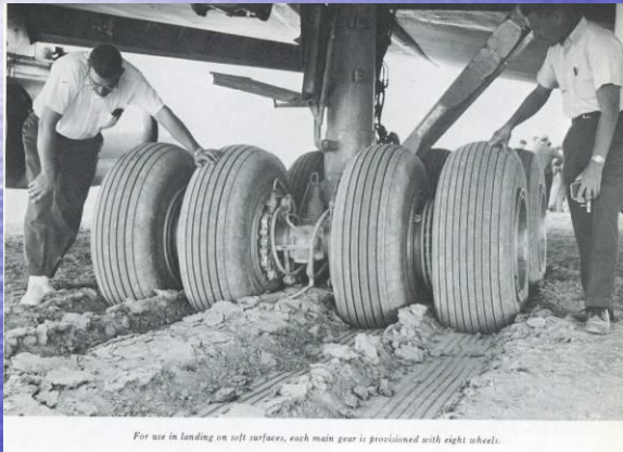
For use in landing on soft surfaces, each main gear is provisioned with eight wheels.
